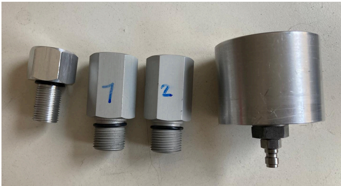
figure 2 - overview testparts with O-rings
