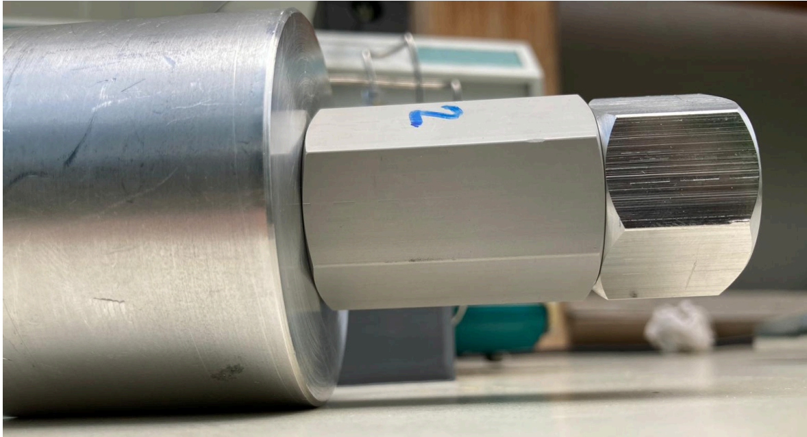
figure 5 - adapter 2: no leakage after 30+ min wait time
