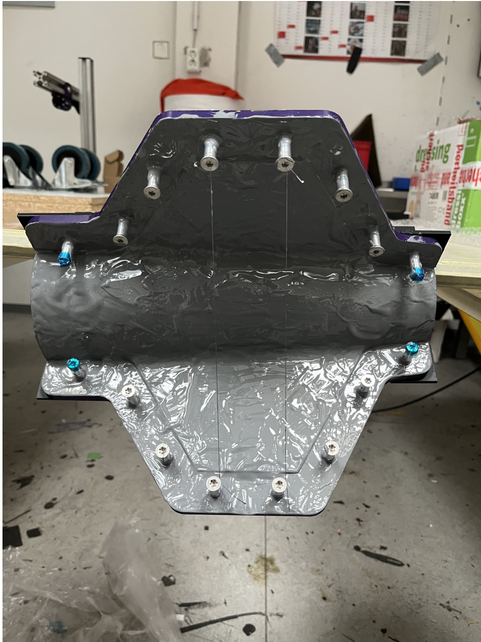
Fig. 2.15: Applying gel coat and molding paste
