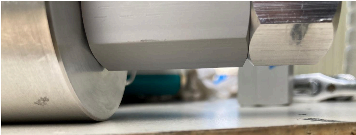
figure 4 - adapter 1: no leakage after 30+ min wait time
