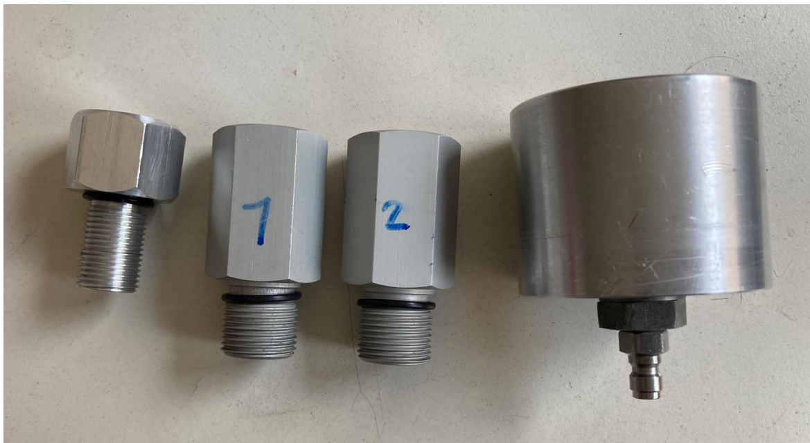
figure 2 - overview testparts with O-rings
