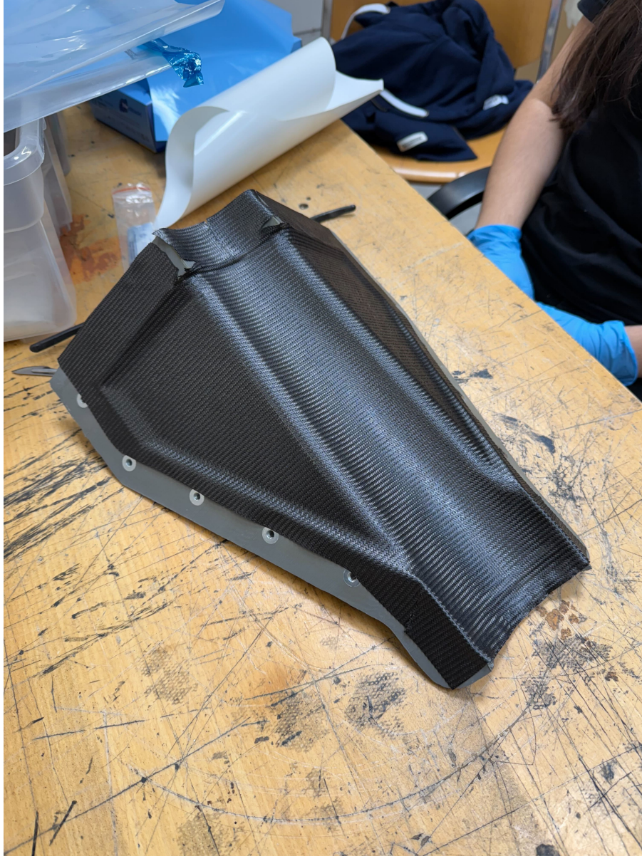
Fig. 2.14: Laminating a fincan segment into our in-house manufactuerd mould
