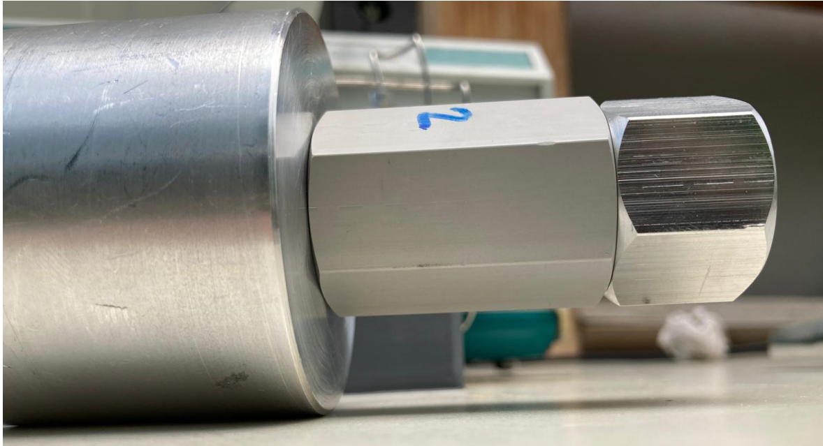
figure 5 - adapter 2: no leakage after 30+ min wait time
