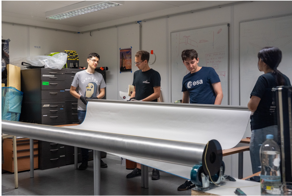
Fig. 2.11: Laminating the body tube
