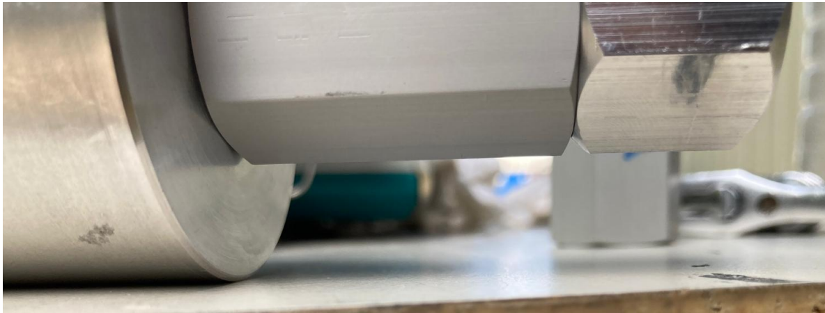
figure 4 - adapter 1: no leakage after 30+ min wait time
